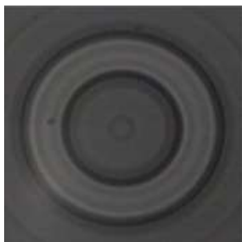
Figure 1. Infrared image of a typical VCSEL oxide aperture used in this study. The P-I characteristics of a similar device is shown in Fig. 2.
