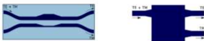
Fig 1: Examples of different designs of PBS: (a) DC-based PSB with phase control stage and (b) 1 × 2 MMI-based PSB.
