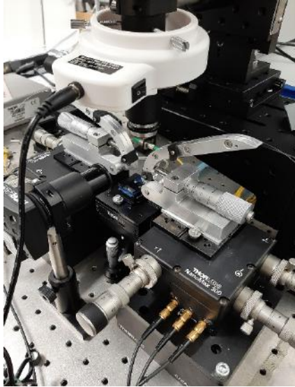
Figure 1: Photograph of passive building block test bed including semi-automatic alignment.
