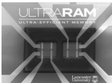
Two 2x2 (4-bit) ULTRARAM™ arrays with 20 nm feature size.
